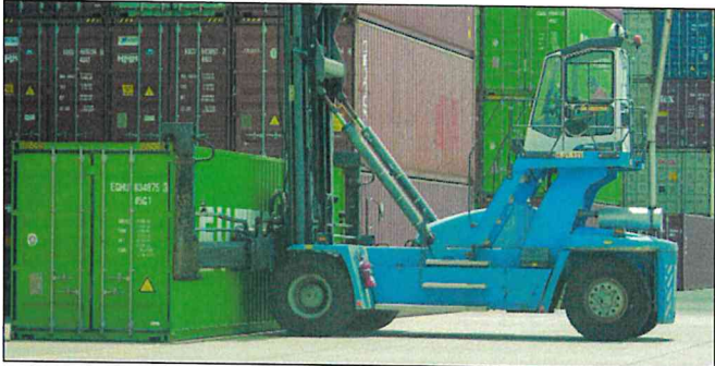
Photo of a toplift lifting shipping containers at Dillon's Inland Port. Photo By Landry Collins/The Dillon Herald
